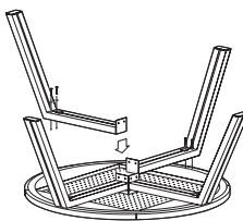
2. Put the four legs in place, with the welded plate facing the centre. Fasten the legs by means of the 8 long bolts and the flat washers. Do not tighten the bolts completely at this stage!
