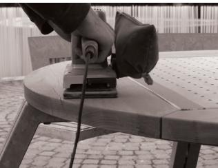
Now sand the tabletop. Make sure the hand sanding machine is held parallel to the tabletop. Do not limit the sanding to the damaged parts, but sand the entire tabletop to obtain a uniform result.
