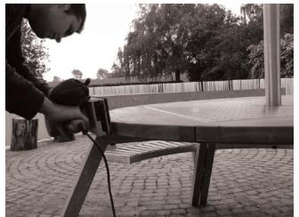
Use 80 grit sanding paper and start with the vertical part of the tabletop. Hold the hand sanding machine parallel to the table's edge. Lightly sand the edge until smooth.
