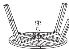
3. Place the central cube in the middle of the table between the four legs. The cube must be positioned with the completely open side facing the tabletop. Fasten the cube to the legs using the 8 short bolts and nuts. The nuts must be put on the inside of the cube. Do not tighten the bolts completely at this stage!
