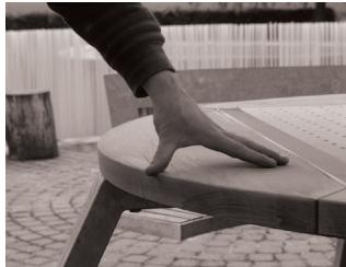
To avoid burrs, sand the top edge of the tabletop until smooth. Sand this part by hand. Upon removal of the burrs, you can, depending on the desired finish, treat the table with hardwood oil.
