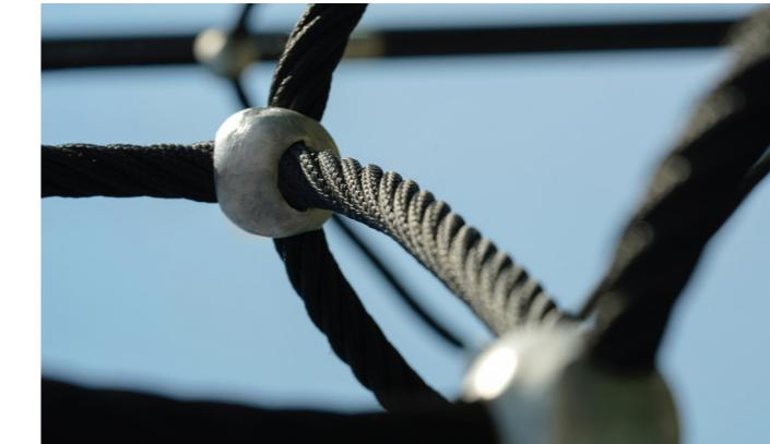
**Single-casing aluminum cast connectors are compressed with 300 tons to avoid moving and premature wear. Ball knot "connector" is shapely and pleasant to grip with no sharp angles or edges.**
