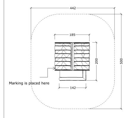
Plan, safety zone (no safety surfacing ar required)
