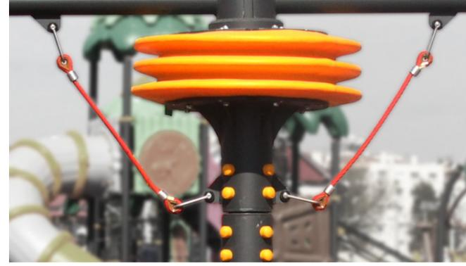
**Cardan mechanism is designed to allow 360-degree rotation and a maximum of 10 degrees of tilting in all directions. To cover the motion system detail, an elastic bellows produced by rotation technique from AFFINITY material will be used.**
