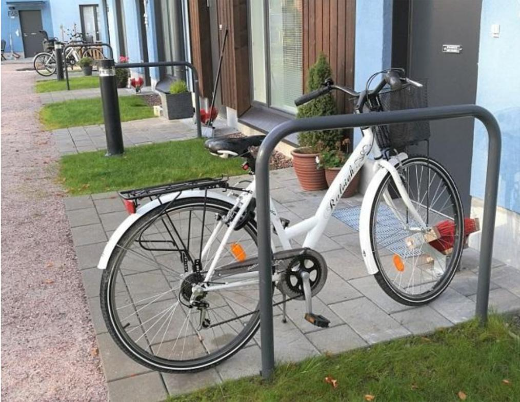
You can lock your bicycle from it's frame to Svallet bicycle stand. The design is simply and smooth so it fits most environments. One Svallet takes two bicycles, one on each side, and recommended free space between stands is 80-100 cm leaving 40-50 cm space for each bicycle. Svallet has two installation versions; deep mounting with wet concrete and surface mounting with fixing plate to be bolted on concrete or asphalt.
