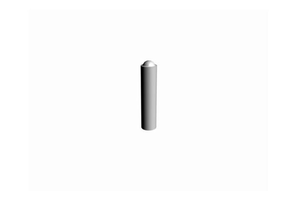
Bollards for roads and public squares. Cylindrical bollards for communal areas where pedestrians and drivers share the same space. The bollard is steel, 750 mm high and c-c 220 mm. Designed for poured foundations.
