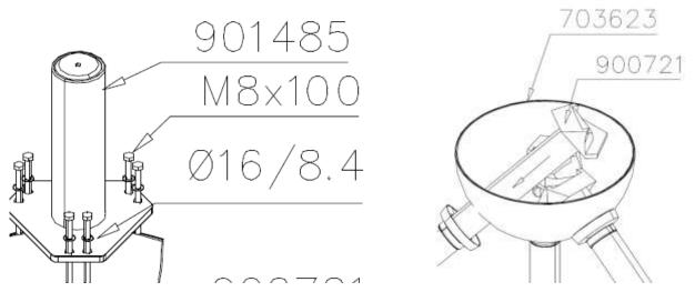
Remove the branch/branches you need to replace the spheres. The branch can be slid up after the allen screws at the aluminum flanges are removed (picture below).
