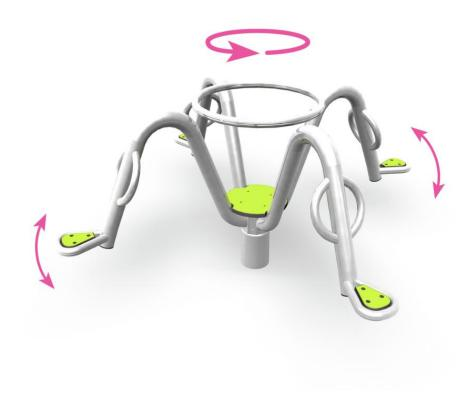
Rotating play equipment with seats for four persons. The seats rotate around a pole and move up and down. The seats are located at a height of 440 mm. A round plate in the middle of the equipment provides space for standing. The small diameter of the equipment prevents the rotating speed getting too high, and therefore the equipment does not need a braking system. Whirling around in the play equipment offers children a fun way of developing their sense of rhythm and balance.
